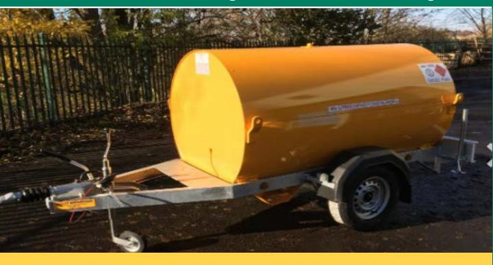
**CHASSIS:** Constructed from 100 x 50 RSC fully welded with front standing plate and 'A' frame drawbar
