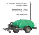
If a 110 V, 32 A power supply with a motor-rated MCB is not available (NB: a 110 V site transformer with thermal cut-out will not work), then we can offer a 5 kVA transformer complete with motor-rated MCB. This transformer will require a 240 V, 16 A power supply socket.
