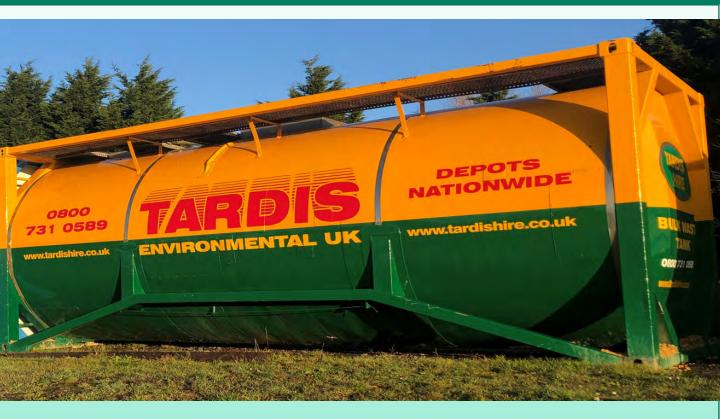
The surface in which the iso tanks are to be situated must be able to sustain the weight of the iso tank when full. Please bare in mind iso tanks when full of liquid range from 27 ton up to 35 ton based on the iso tank size requested
