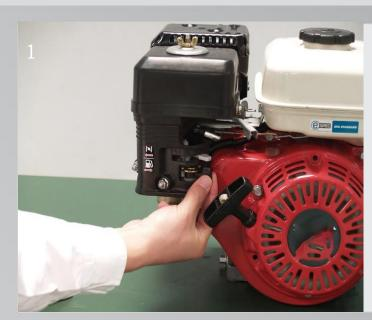
Turn the fuel valve lever to the ON position.
