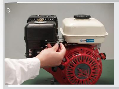
Move the throttle control lever slightly to the left.
