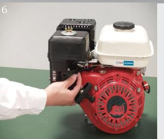
Gradually move the choke lever to the OPEN position as the engine warms up.
