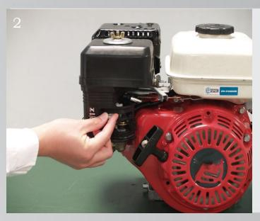
Move the choke lever to the CLOSED position.
