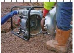
\*\*\*\*These pumps aren't compatible with E10 petrol and must be used with E5 petrol only Any call outs in relation to this will be chargeable to the customer, as we would need to drain and replenish each engine with new Super unleaded to run correctly\*\*\*
