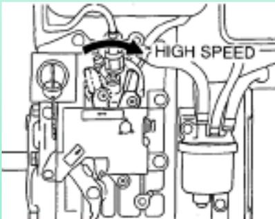
Once the engine is running, start the engine with the speed adjust lever at LOW speed and allow the engine to warm up. Increase the speed by moving the level to the right
