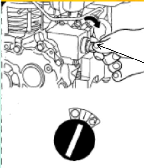
Do not run the starter motor for more than 5 seconds
